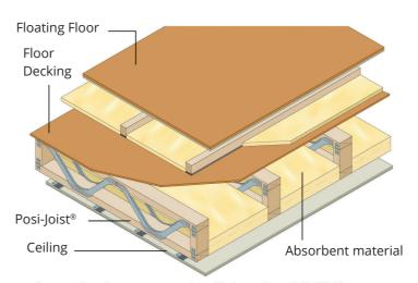
Separating floor construction (Robust Detail E-FT-3)
