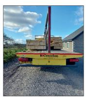
5. The manufacturer will supply Posi-Joists banded in packs (each layer to be banded individually) with yellow banding.
