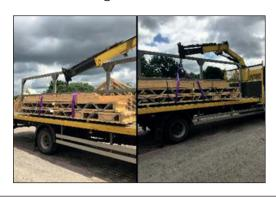
8. Lift slowly to ensure the load is balanced, if not lower down and adjust the slings. Ensure no persons are within the lift area.
