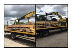
7. Lift slowly to ensure the load is balanced, if not lower down and adjust the slings.
