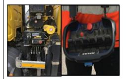
**3.** Bring out the stabilisers fully and attach the foot pads
