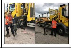
**4.**Wearing of the remote controller is important, the strap needs to be around the neck and over the shoulder and not just around the neck. When just around the neck if you bend the controller will swing away from the body and if not deactivated there is potential for it to knock against something and activate the HAIB. **ALWAYS DEACTIVATE CONTROLLER WHEN NOT BEING USED**
