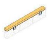
38-75mm wallplate bedded on mortar and fixed to gable restraint brackets with 3.5x40mm wood screws (2 no. per bracket).
